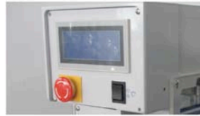
PLC Control Touch Screen Panel
